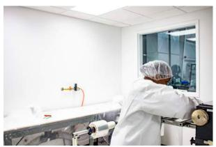
hydraulics are used instead, any fumes are removed. Because the housings that hide moving parts may obscure sightlines, some cleanroom die cutting equipment uses machine vision.
